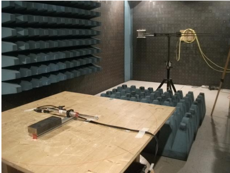
Photo test set-up for frequency up to 1 GHz
