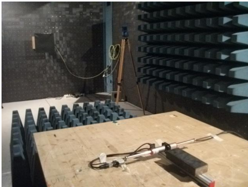
Photo test set-up for frequency above 1 GHz
